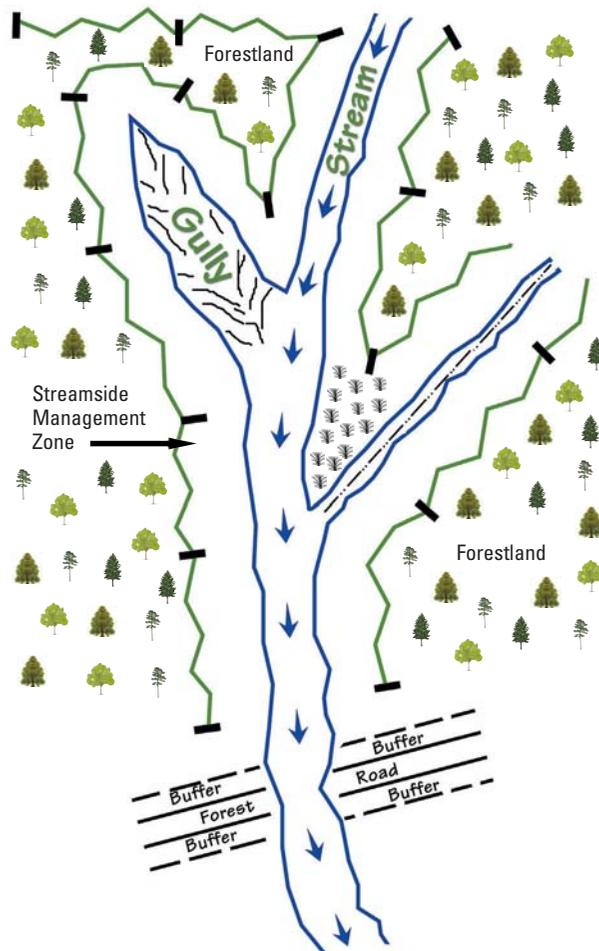
Establishment of SMZs and water diversions are important for water quality when installing firebreaks near streams, gullies, wetlands, and roads. Water diversion placement and SMZ widths are determined by slope and stream type.
