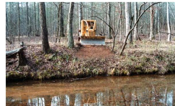
Ranger back blades with dozer to minimize soil disturbance in an SMZ.
