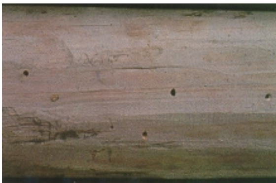
Fig. 10. Many of the wood boring beetles produce exit holes that are similar in size and shape. The holes in this photo were made by at least two separate species. (GFC Photo)
