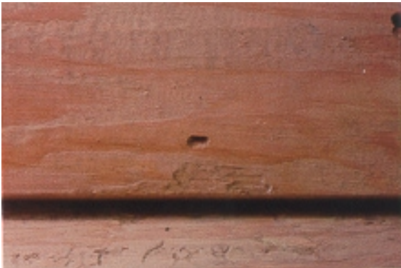
Fig. 8. Exit holes made by adult wood boring beetles may be oval to flattened in shape depending on the species. (GFC Photo)
