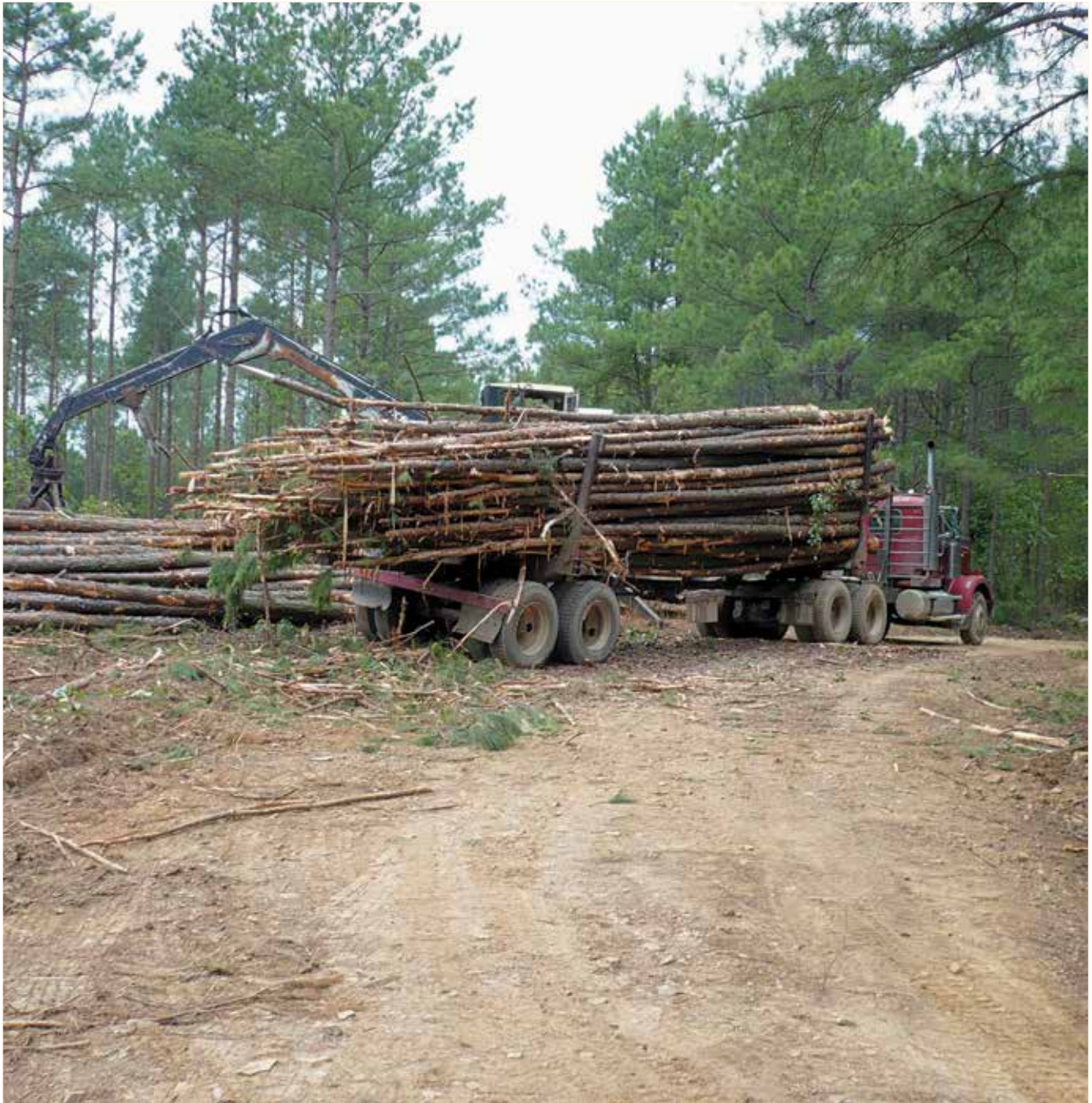
Log truck with pole trailer loaded with tree-length loblolly pine pulpwood.
