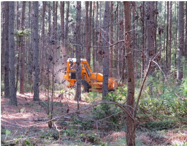
Above left: A Georgia Forestry Commission brushcutter reducing fuel in a pine stand. Above right: a Front mounted drum type mulcher/mower removing understory vegetation and ladder fuels. This type of fuel reduction work in WUI is practical when prescribed fire is not possible.
