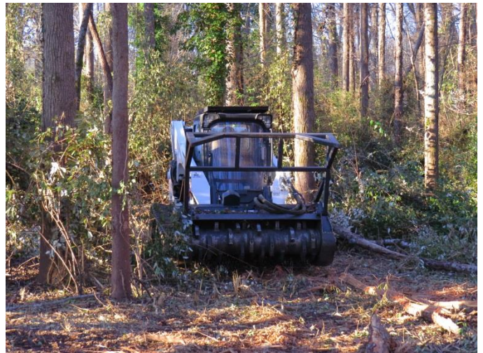
Above left: A Georgia Forestry Commission brushcutter reducing fuel in a pine stand. Above right: a Front mounted drum type mulcher/mower removing understory vegetation and ladder fuels. This type of fuel reduction work in WUI is practical when prescribed fire is not possible.
