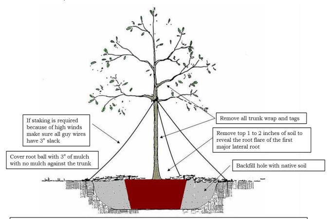
Excavate hole 3X the diameter of the container and 1" to 2" slightly shallower than the depth of the soil inside. Excavate wider in poor soils or heavy clays. Allow 640 sq.ft. of open soil surface area for each overstory tree and 25' – 40' spacing between trees with a minimum of 8' wide planting area. / Allow 400 sq.ft. of open soil surface area for understory trees and 20' spacing between trees with a minimum 6' wide planting area. (Rev. 9/3/208)
