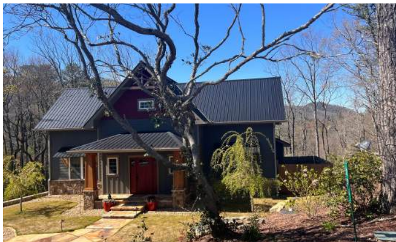
Some homes in Rabun County have exemplary defensible space with mowed grass near structures, trees limbed and not overhanging roofs, non-flammable barriers, within Zone 1.
