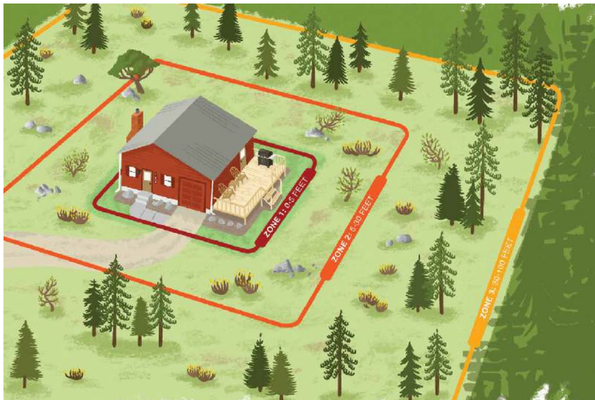
Figure 3.a.2. Home ignition zones recommended by Firewise.org. Using ignition-resistant building materials and removing burnable fuel around primary structures, outbuilding such as sheds, and campers / RVs is crucial for increasing your home’s chance of surviving a wildfire and creating safe conditions for wildland firefighters.
