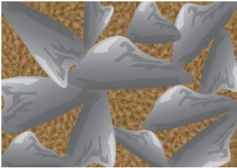
Conceptual diagram of structural soil (Bassuk, 2007)
