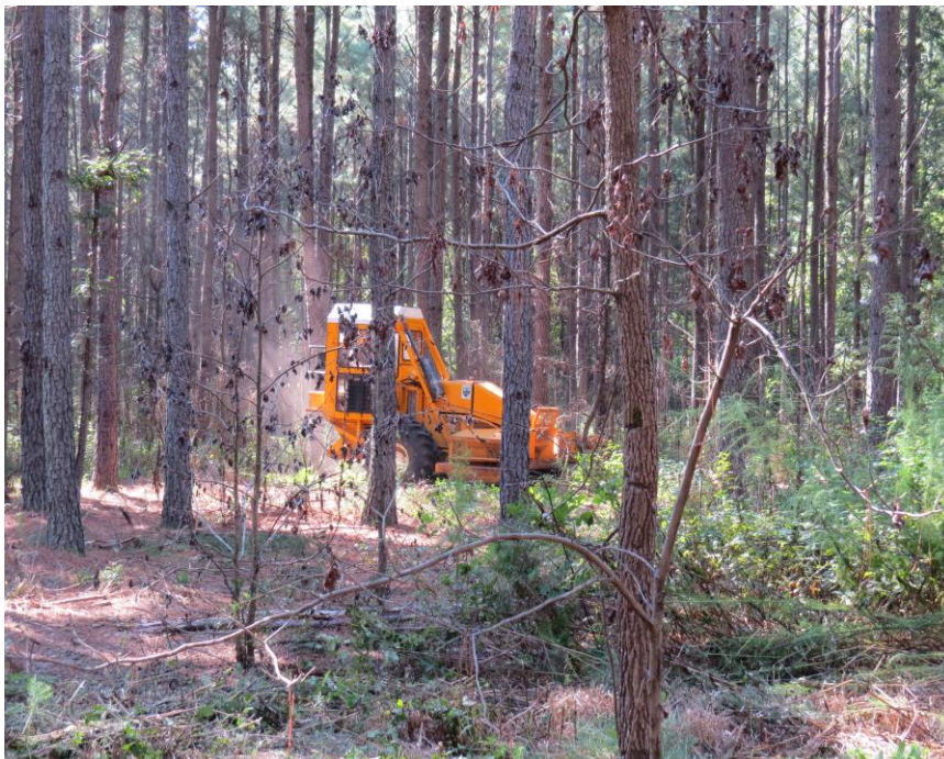
Equipment is available that can be used to mitigate hazardous forest fuels in areas where burning and prescribed fire may not be practical. Pictured here is a Georgia Forestry Commission masticator mowing understory vegetation in a thinned loblolly pine stand.
