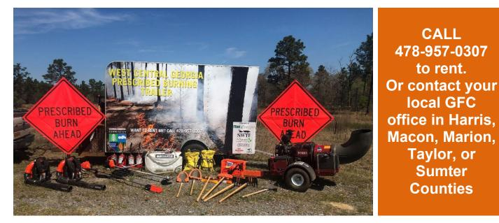
Prescribed burn trailer equipment includes: drip torches, fire rakes, Pulaski, forest shovel, Mcleod, water tank & pump, pole saw, brush cutter, bladder bags, pull-type blower, chainsaw, forestry wedge, saw safety kit, smoke ahead signs, wiring adapter and ramps.
