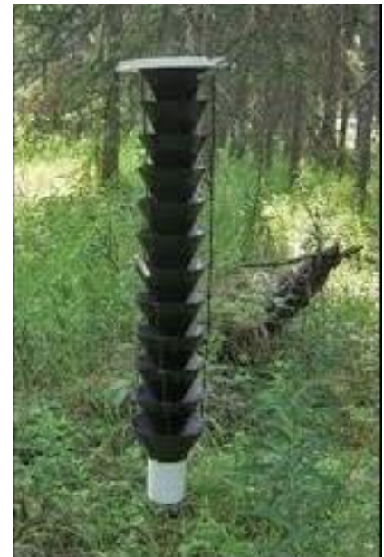
Figure 1: Lindgren funnel trap used to monitor southern pine beetle populations.
