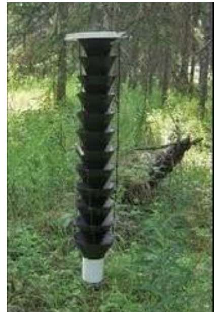
Figure 1: Lindgren funnel trap used to monitor southern pine beetle populations.
